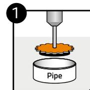
1 Insert the EzyGrind inside PVC pipe. Begin cutting by pushing firmly against the pipe wall until it cuts through
