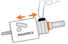
To remove the Hole Saw to use another diameter, just push the button and exchange the Hole Saw. Slide on another Hole Saw and you are ready to go.
